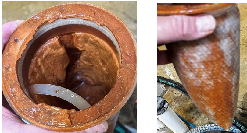
Figure 12. Bag filter at end of study
