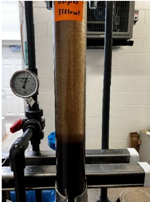
Figure 18. Solids during backwash
