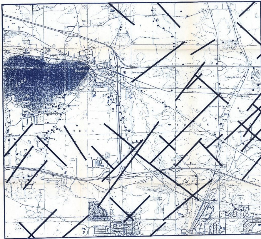
CONTOUR INTERVAL 10 FEET NATIONAL GEODETIC DATUM 1983 FRACTURE TRACE MAP TOWN OF PEWAUKEE, WISCONSIN • Dolomite Well • Sand and Gravel Well / Fracture Trace MAP 4 Ted Zorlich & Associates, Inc. November, 1995
