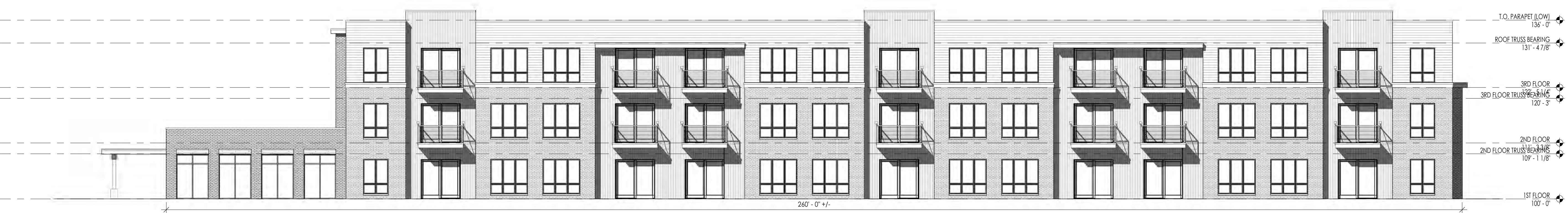
11 BUILDING A1 NORTH ELEVATION SCALE: 3/32" = 1'-0"
