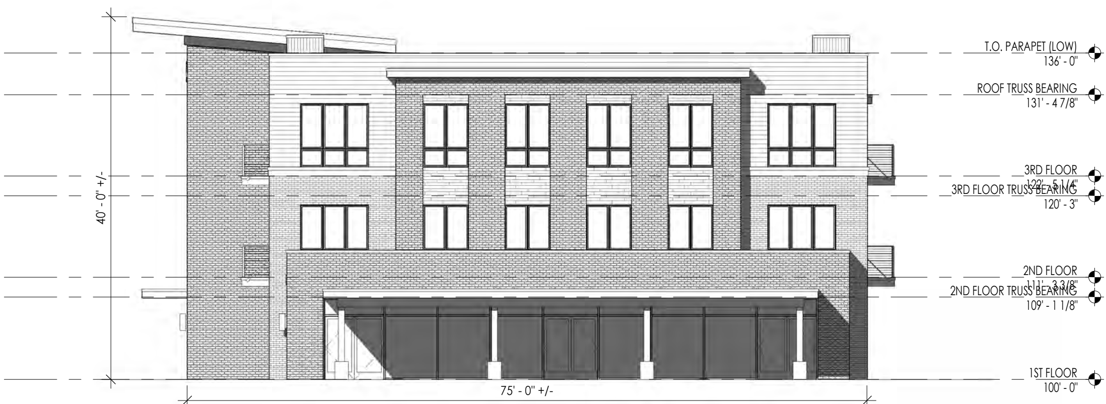
4 BUILDING A1 EAST ELEVATION SCALE: 3/32" = 1'-0"
