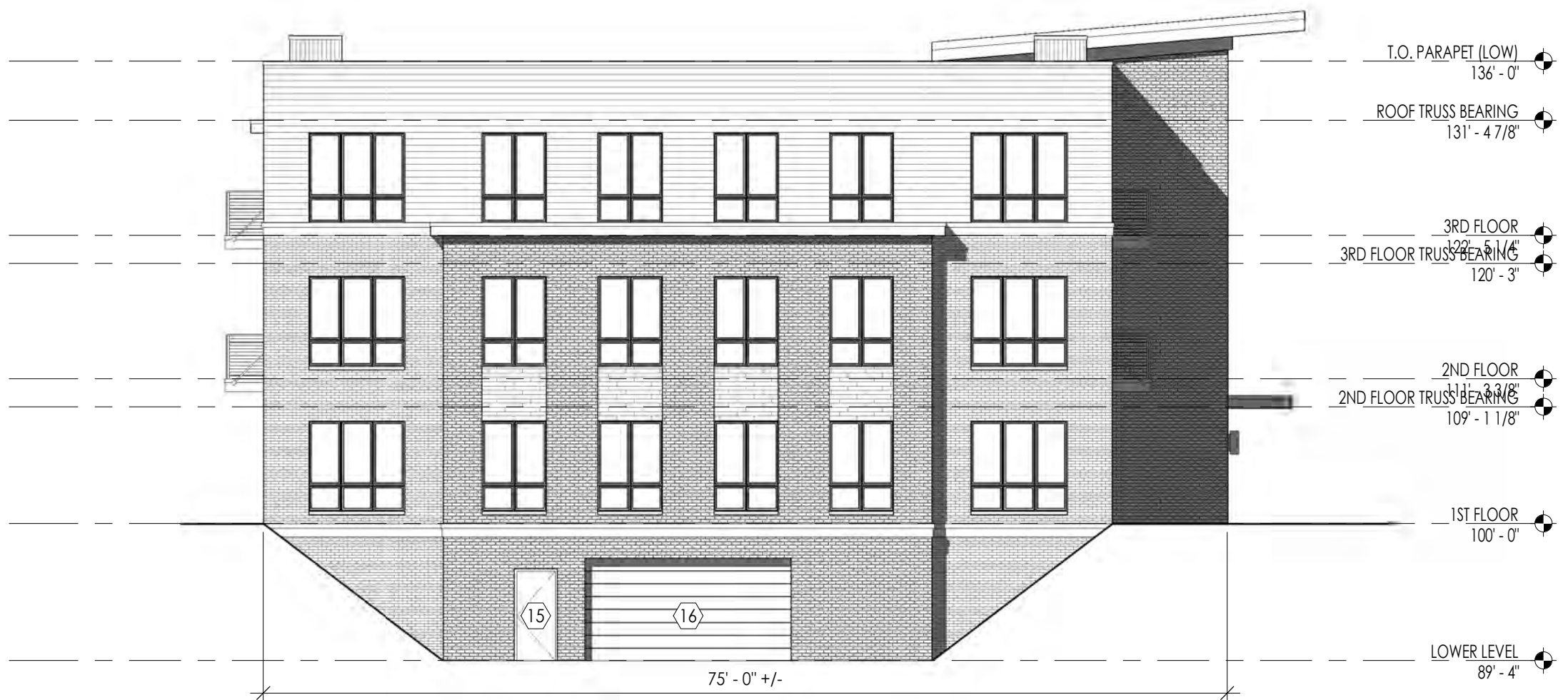
3 BUILDING A1 WEST ELEVATION SCALE: 3/32" = 1'-0"
