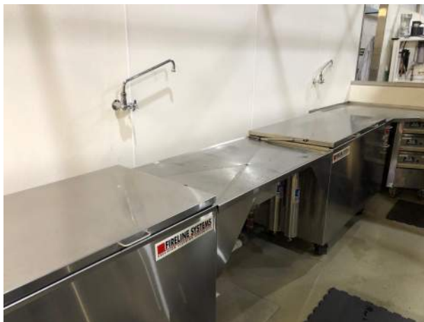
Paul Davis - Pre-Soak and Ultrasonic Station
